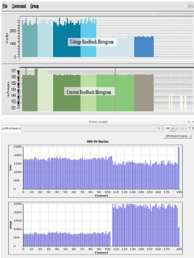
FIG. 3. Voltage and current values for all detectors, as seen from Tcl/Tk (top) and CSS (bottom). Each detector is represented by a different color on the Tcl/Tk screen.
